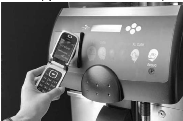
Figure 4. An NFC-enabled mobile phone with the corresponding payment application simulates a contactless credit or debit card [8]
