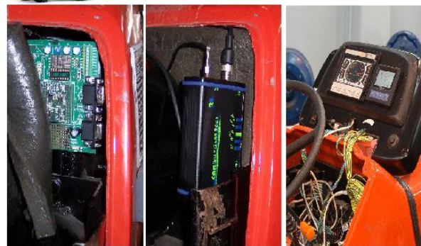
Fig.6: System for service load data acquisition trough CAN bus: top – configuration of the system, bottom left – EM built in the tractor; bottom middle – GPRS modem built in the tractor, bottom left – installation of the WD unit.
