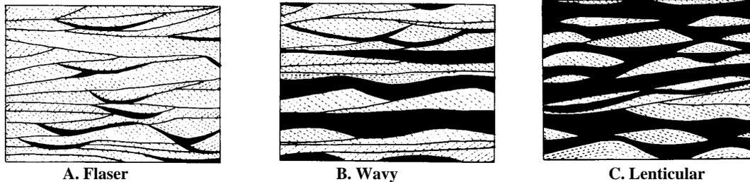
Figure 2-7 Flaser, Wavy and Lenticular Bedding.
