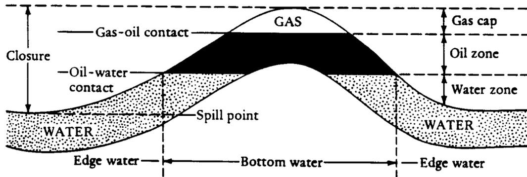
Figure 4-3 Cross-section Of A Simple Anticlinal Trap
