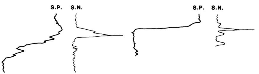
Figure 5-9 Sedimentary Environments from the SP Curve
