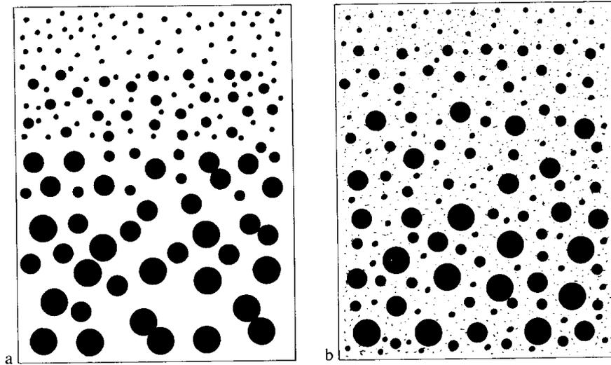
**Figure 2-4** Two basic types of graded bedding; a) no fines and b) fines present as matrix.
