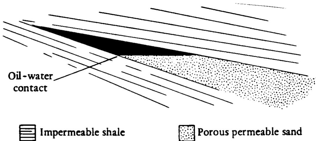
**Figure 4-8 Example Of A Lenticular Trap**
