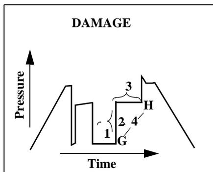
With some exceptions, a damaged zone will be indicated by the configuration of the shut-in curve (GH). Specific indicators are a very sharp rise after the final flow (1), a short curve radius (2), a reasonably flat slope (3), and a high differential pressure between the final flow and final shut-in (4).
