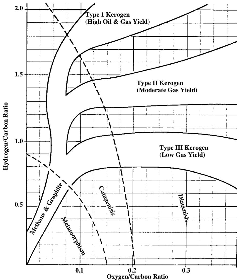
Figure 7-1 Van Krevelen Diagram Showing the Thermal Progression of Kerogen
