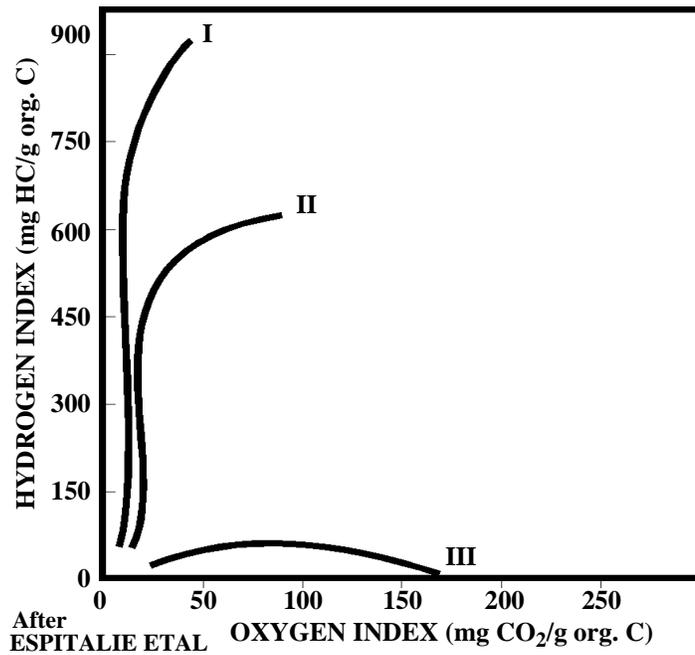
Figure 7-8 Hydrogen Index vs Oxygen Index
