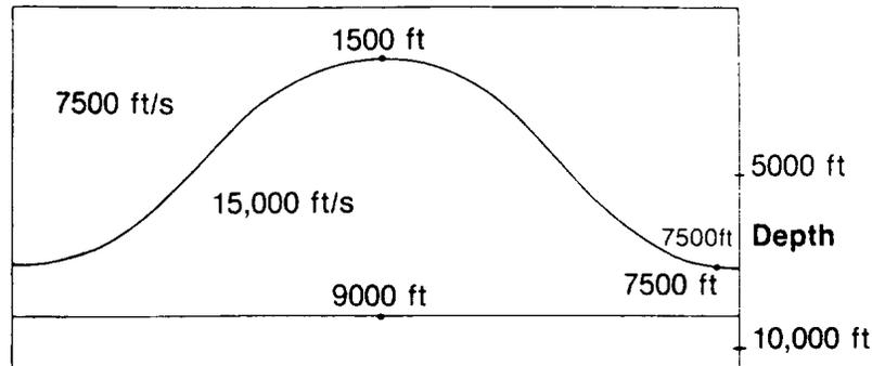
**Figure 6-14** The salt in [Figure 6-13](#), having a travel time of 15,000 ft/s, causes the seismic wave from the base of the dome to return to the surface faster than the surrounding rock, causing the reflection to appear higher than it actually is.
