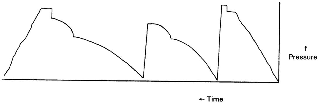
**Figure 8-4 Double Shut-in Pressure Record**
