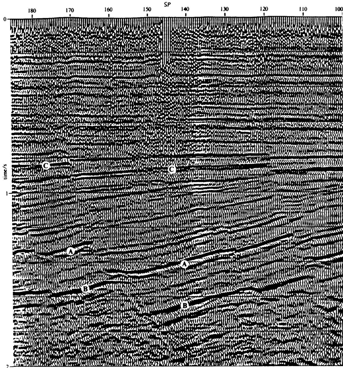
**Figure 6-12 Seismic Section with a Fault Cutting Several Reflectors**
