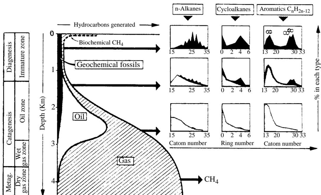
Figure 7-3 The Oil Window, and General Scheme of Hydrocarbons Produced
