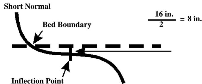
**Figure 5-4 Bed Boundary Location Using the Short Normal**
