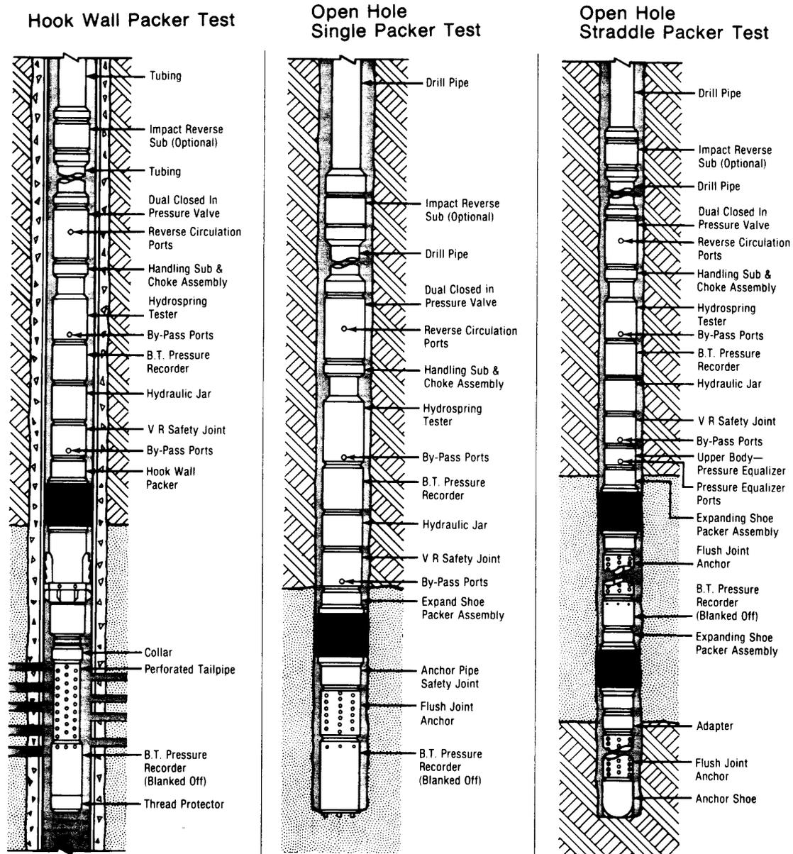
Figure 8-1 Three Basic DST Assemblies (from Halliburton Services)
