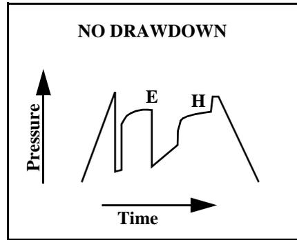
However, where the difference between the initial shut-in pressure (E) and the final shut-in pressure (H) is less than two percent, as it is here, the chart would suggest not only high permeability but also a potentially commercial reservoir.
