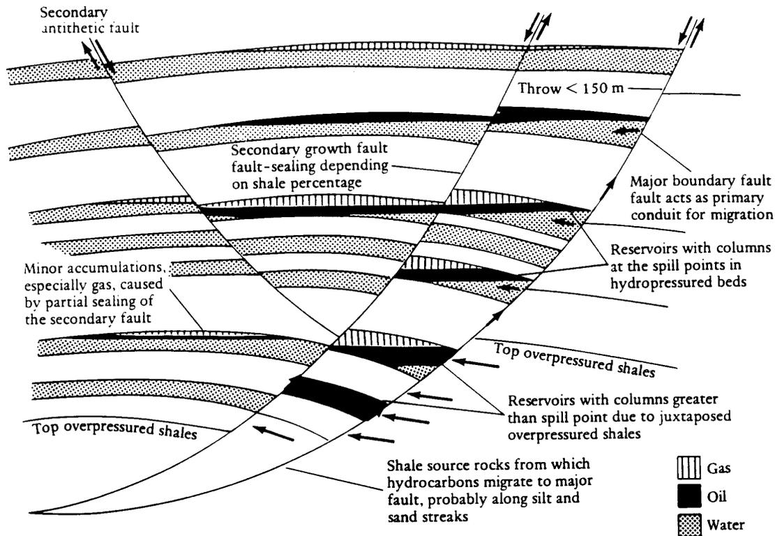
Figure 4-6 Accumulation Of Hydrocarbons (And Abnormal Pressure) Around Growth Faults
