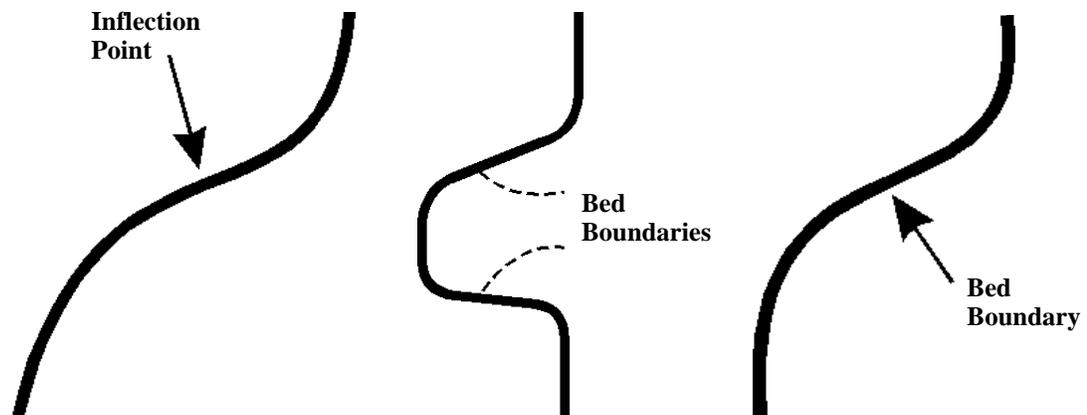
**Figure 5-3 Location of Bed Boundaries Using the SP Curve**
