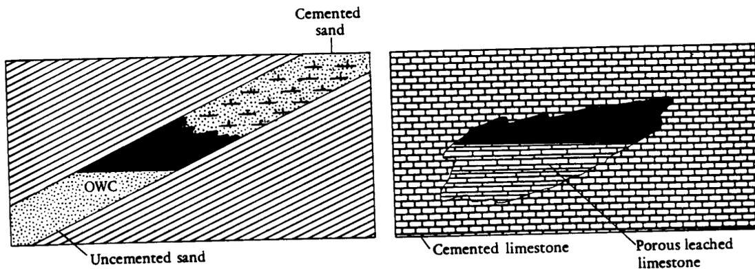
**Figure 4-7 Stratigraphic Traps Resulting From Changes In Their Depositional Environment**
