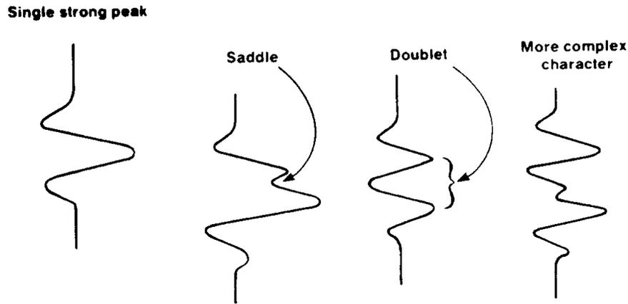
Figure 6-9 Character of Seismic Wiggles
