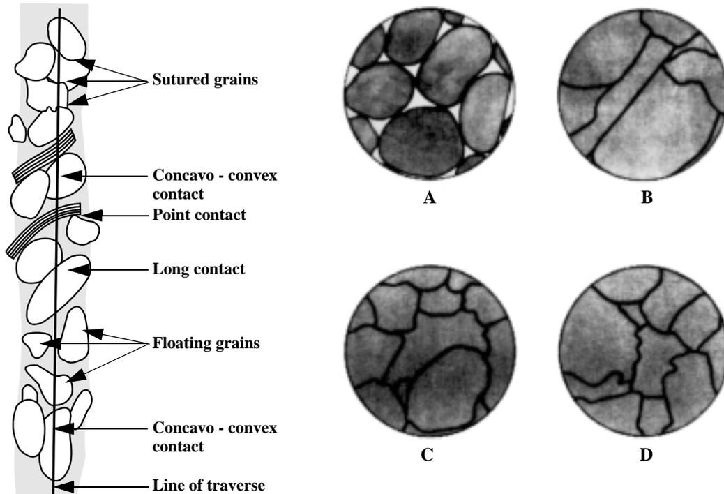
Figure 1-3 Grain Contact Terminology: A) point contact, B) long contact, C) concavo-convex, D) sutured
