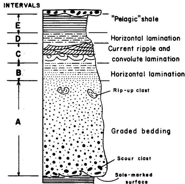
Figure 2-5 Graded bedding in an "ideal" Bouma cycle.
