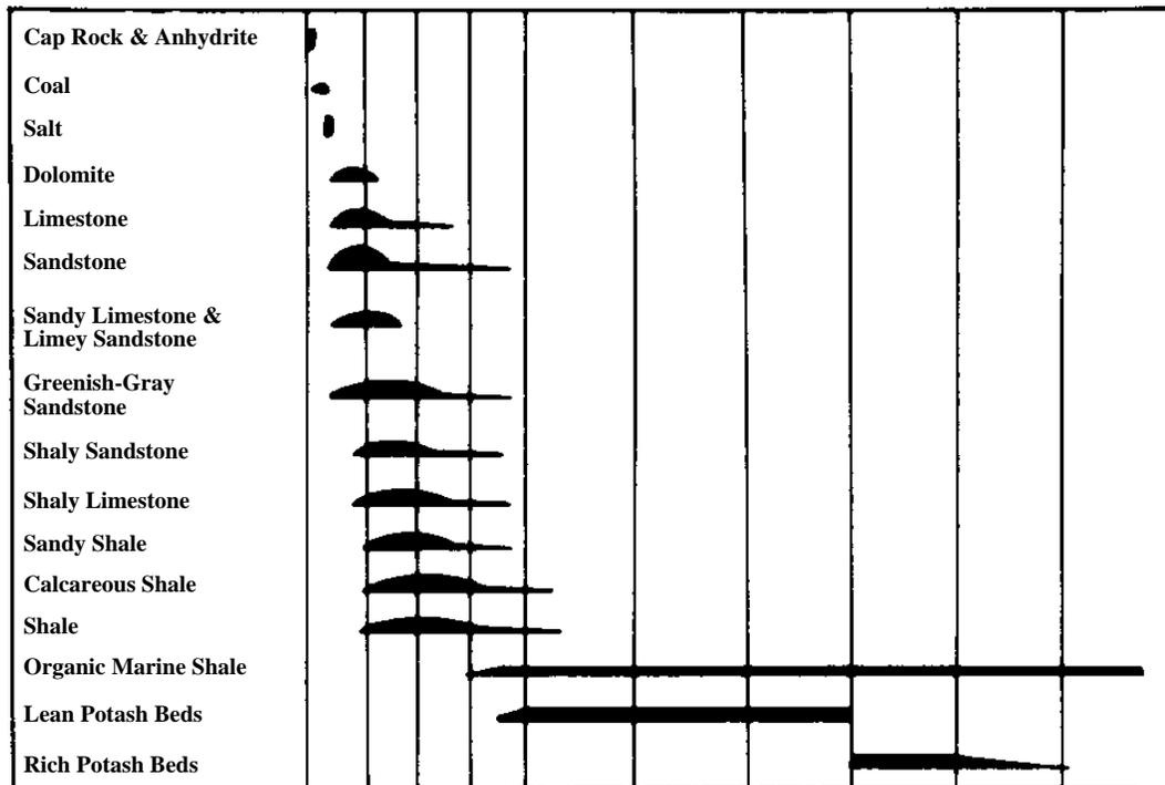
The length of the line denotes the intensity range in API Gamma Ray Units. The vertical width of the line increases with the frequency of occurrence.
