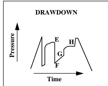
Because the final shut-in pressure (H) is much lower than the initial shut-in pressure (E), this chart indicates that the reservoir tested was “drawn down” considerably (line FG) and may be limited in size.
