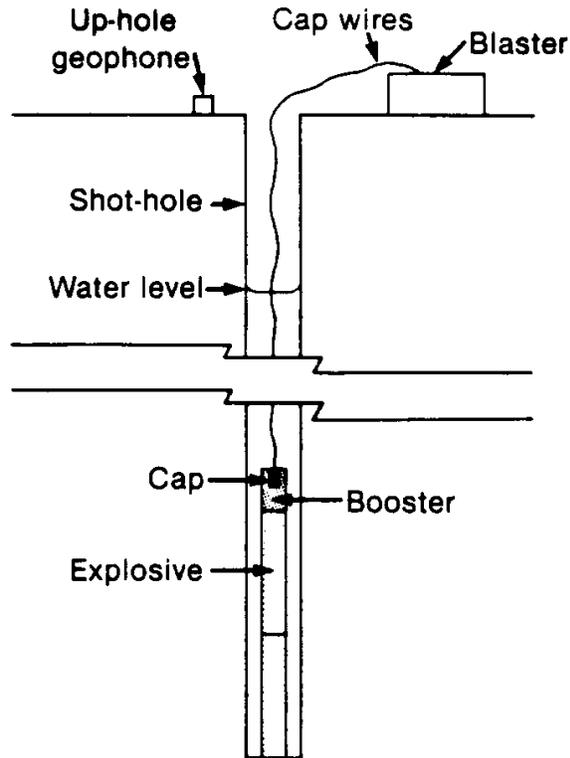
**Figure 6-4 Schematic of an Onshore Shot-Hole**
