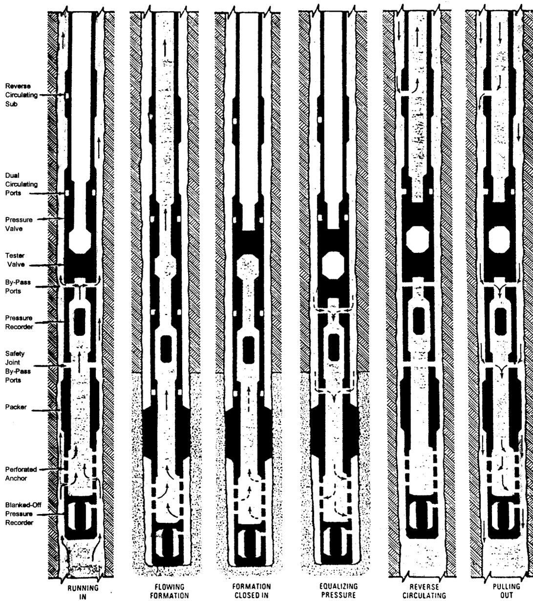
Figure 8-2 TESTING - Fluid Passage Diagram
