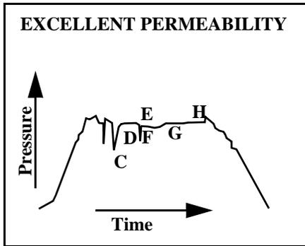
This chart, on the other hand, suggests a zone with high permeability. The shut-in curves (DE and GH) were developed faster, and the flow curves (CD and FG) indicate a high rate of fluid entry to the test tool.
