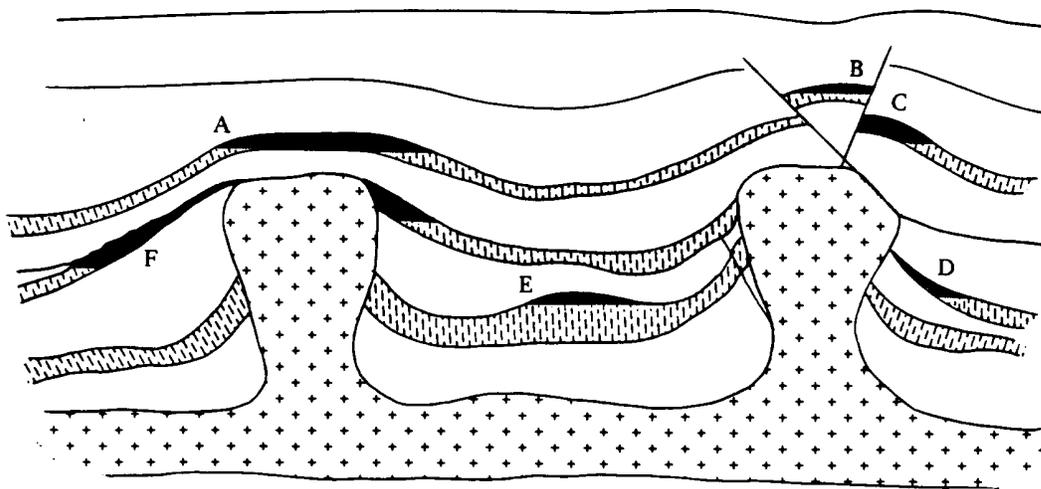
**Figure 4-1 Types Of Traps That Develop Through Salt Movement (A-Domal Trap, B&C-Fault Traps, D-Pinchout Trap, E-Anticlinal Trap, and F-Truncation Trap)**
