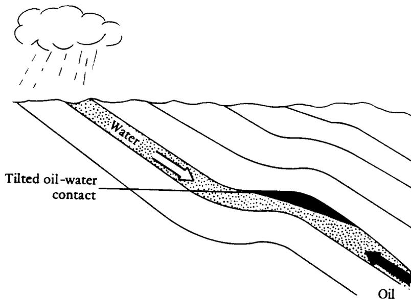
**Figure 4-2 Example Of A Hydrodynamic Trap**
