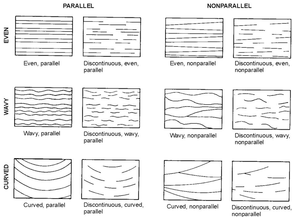
**Figure 2-1** Different shapes that can be acquired by beds.
