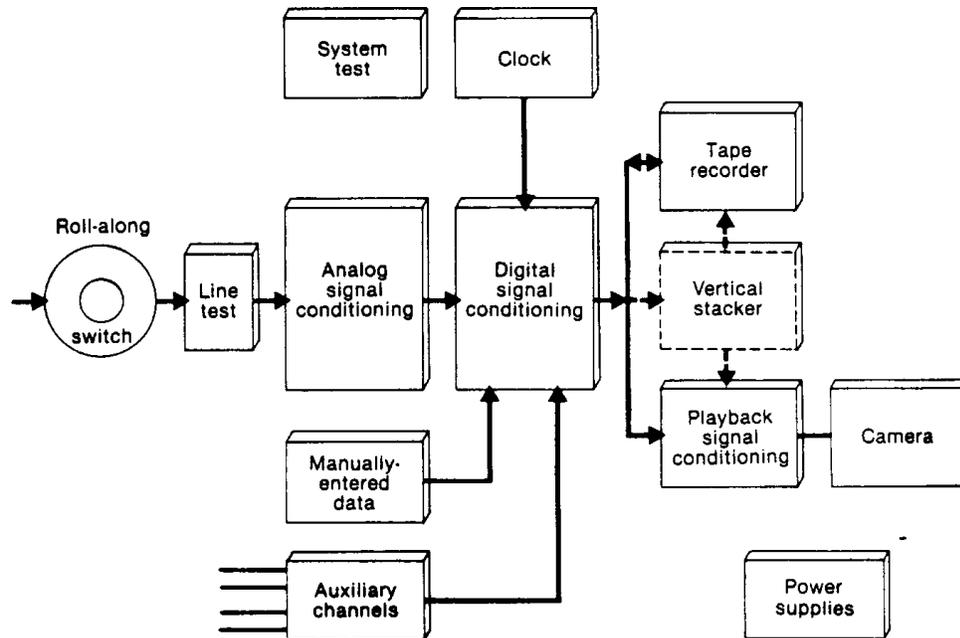
Figure 6-5 Seismic Recording Instrument Layout
