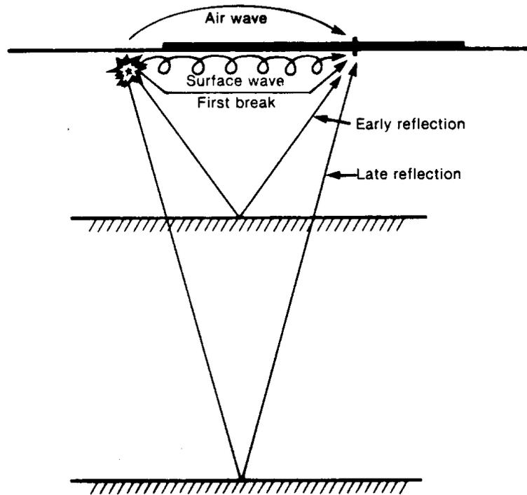
**Figure 6-7 Types of Reflections from a Seismic Shot**
