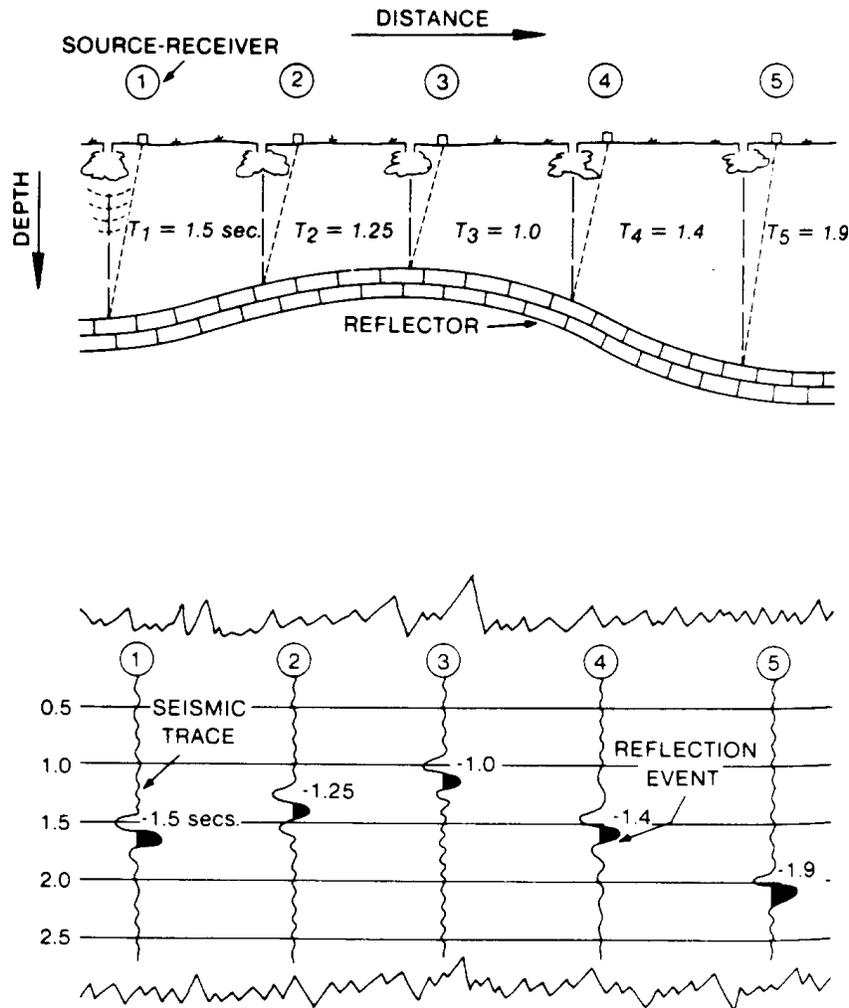
**Figure 6-3 Generation of Seismic Traces**
