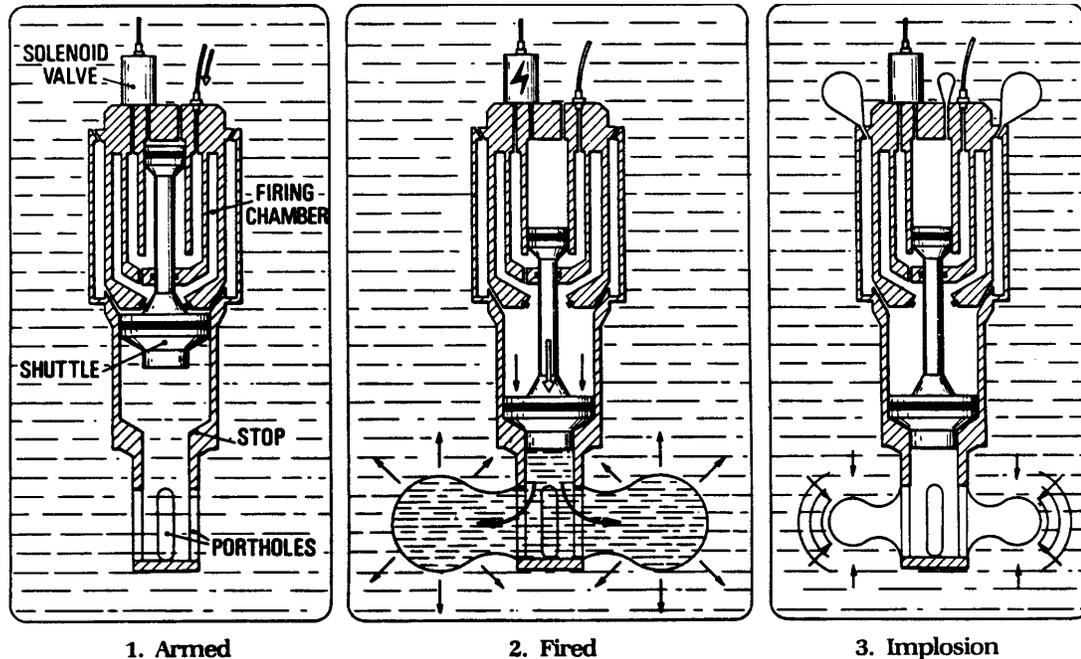
Figure 6-6 Water Gun Operation
