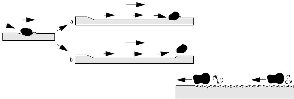
Figure 2-9 The development of a groove mark caused by a moving object.
