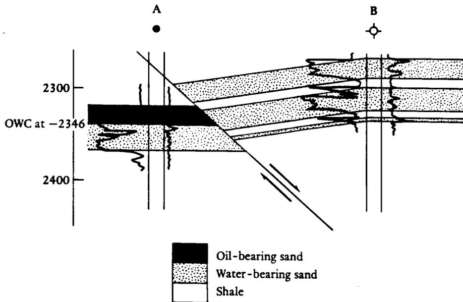
Figure 4-5 Fault Sealing, Caused By Impermeable Material, Along A Permeable Sand
