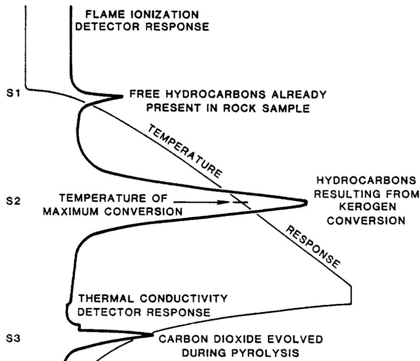
Figure 7-5 Source Rock Evaluation by Pyrolysis
