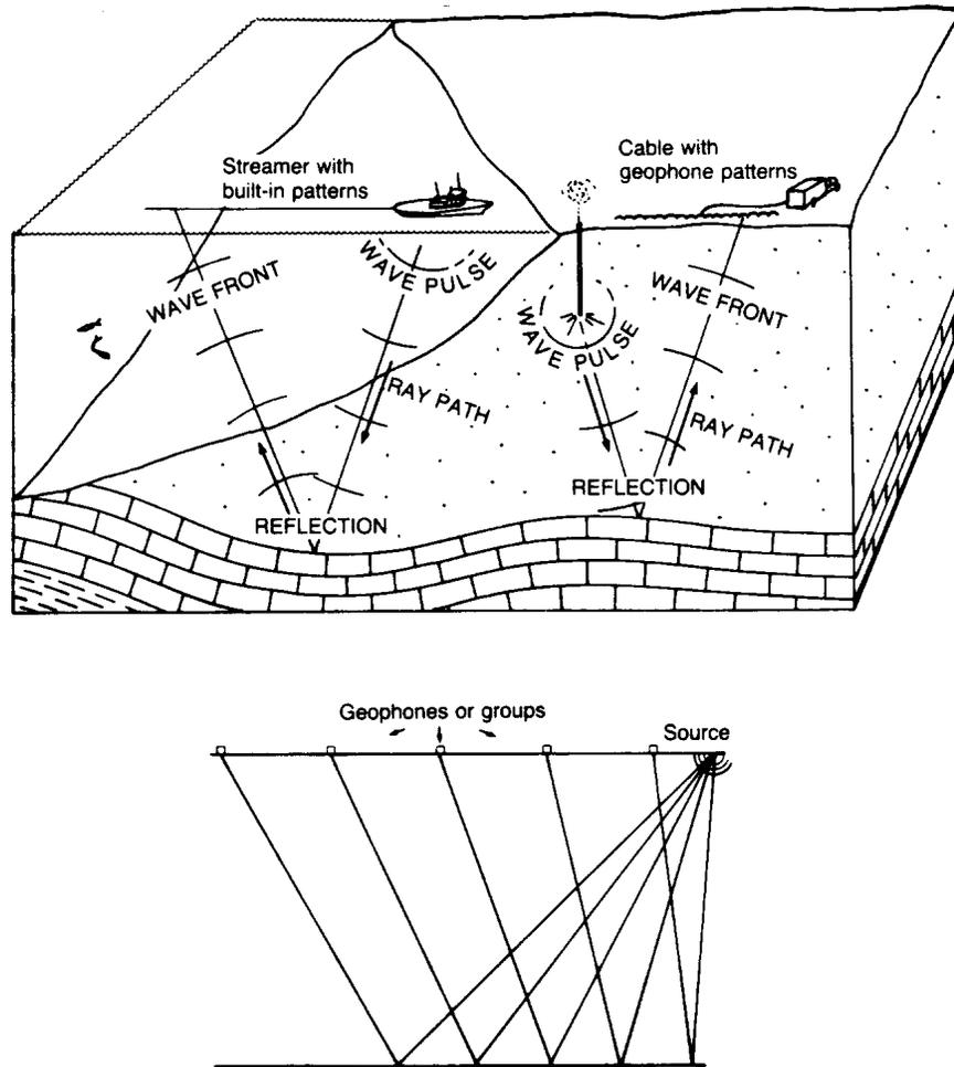
**Figure 6-1 Generation of Seismic Reflections**
