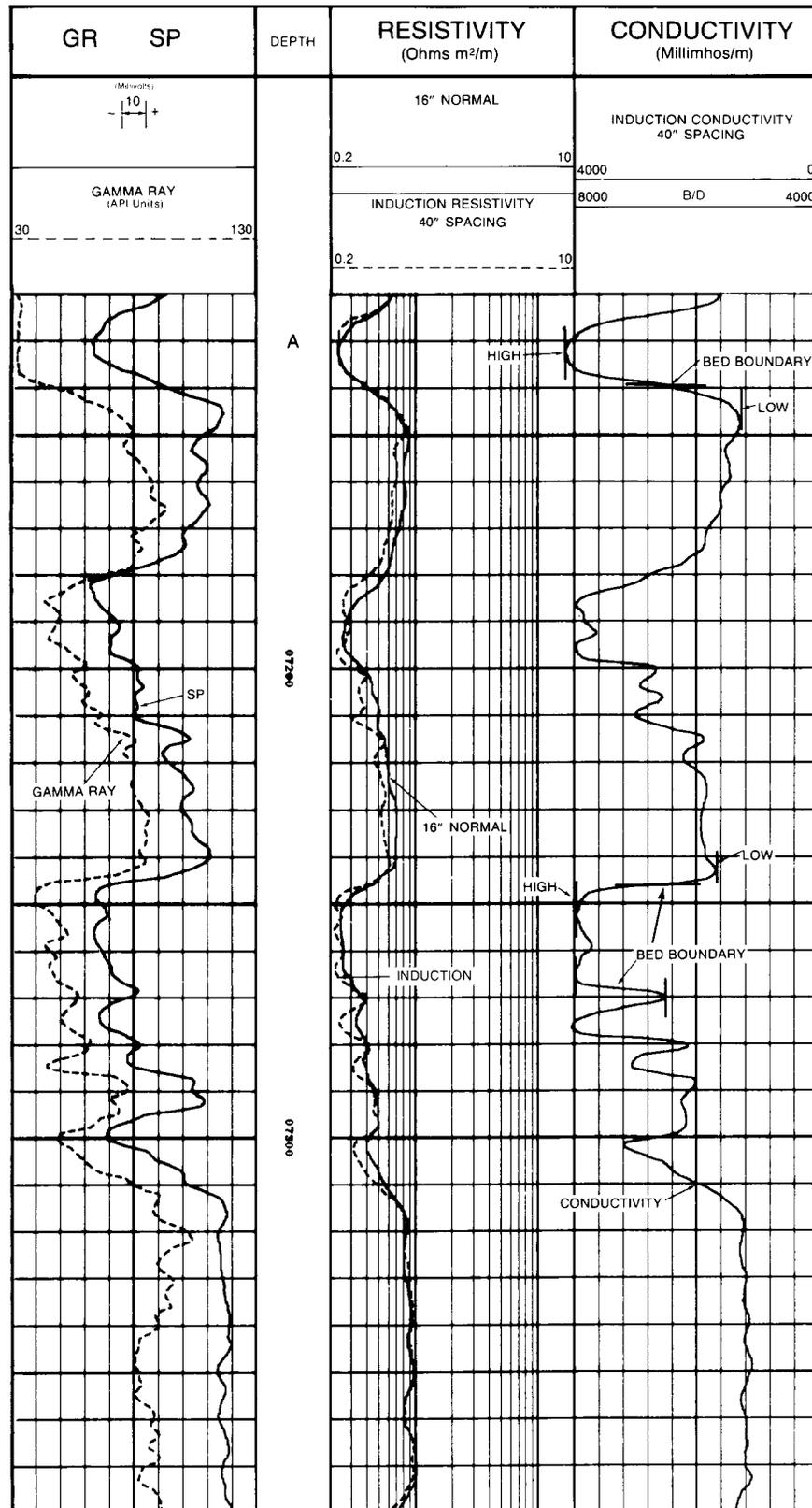
Figure 5-5 Bed Boundaries From Conductivity Curve
