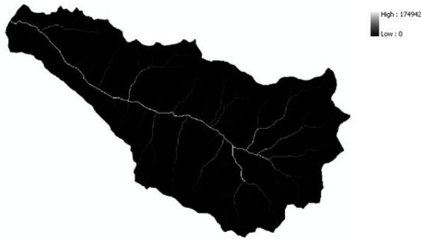
Figure 6. Flow accumulation in the River Banjska basin up to the “Vranjska Banja” HS
