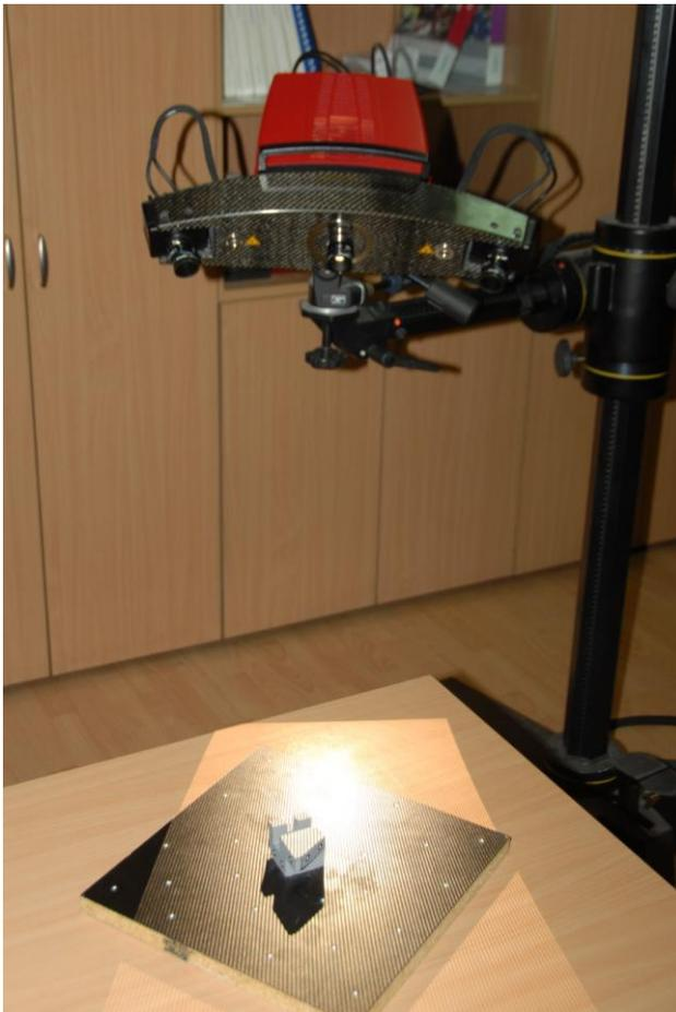
Figure 7. Digitizing of model with high-end industrial 3D scanner ATOS
