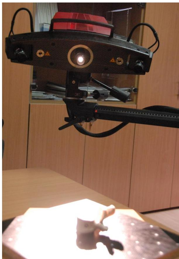
Figure 1. ATOS (Advanced Topometric Sensor) 3D scanner
