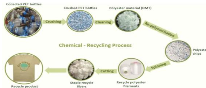
Figure 7. The production process of recycled polyester fiber
