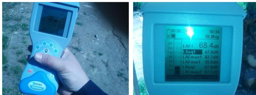
Figure 3. Results from performed measurements of noise in front of the powerhouse
