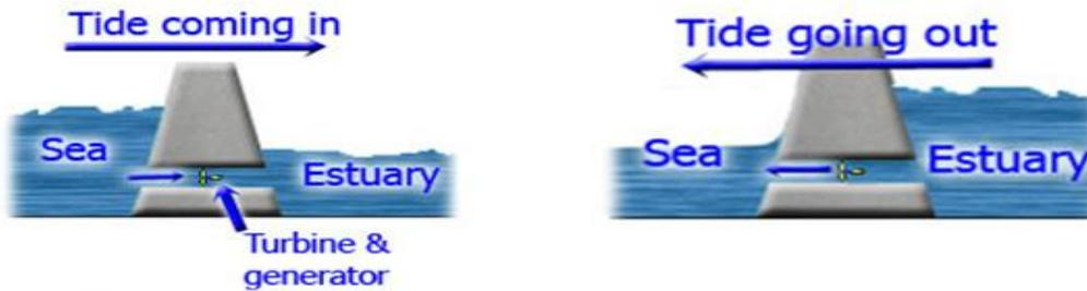
**Figure 1.** Collecting the energy of high and low tide, graphic representation
