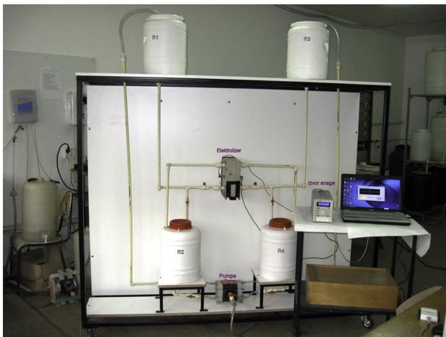
**Figure 1.** Device for electrochemical synthesis of ferrate(VI)
