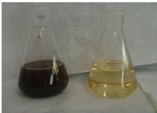
**Figure 3.** Sample of WW from the steam chamber before the treatment and after the second step of the treatment by ferrate(VI)
