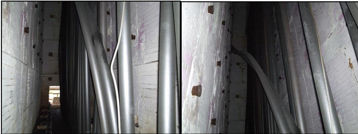
**Figure 2.** Pyrolysis furnace radiant zone - consequence of a high creep rate
