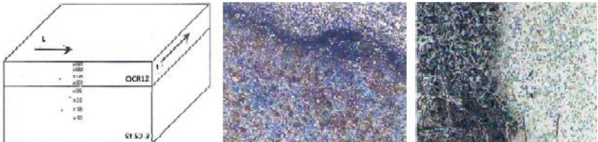
**Figure 3.** Schematic of measuring hardness of HV5, joint boundaries Č0562 (S355J2G-3)-10mm and Č4850 (x153CrMoV12)-3mm. State: explosion welded (1), tempered in furnace (2)
