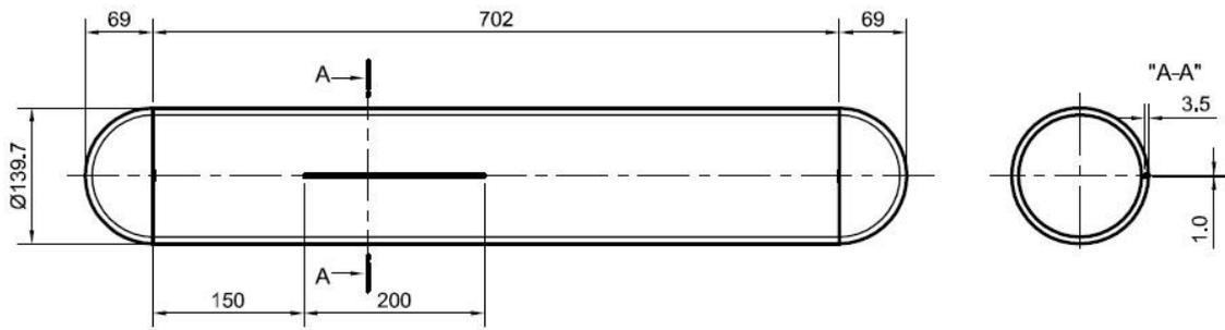
**Figure 1.** Pipe (pressured vessel) with an axial surface crack on the outer surface
