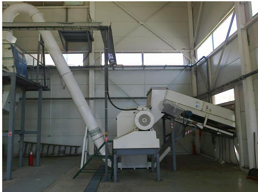
**Figure 2.** Hammer for rough grinding of straw and transport
