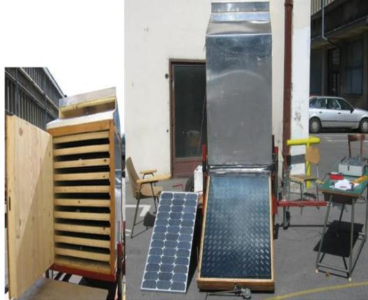
**Figure 2.** Prototype of a module of a mobile universal solar dryer
