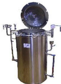
**Figure 4.** Laboratory autoclave
