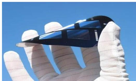
**Figure 3.** Photovoltaic solar cells made by thin-film technology [12]
