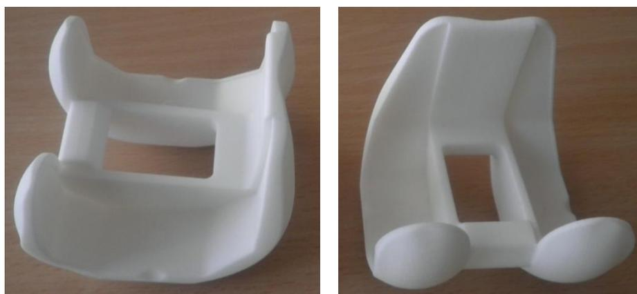
**Figure 2.** The SLS knee implant geometry
