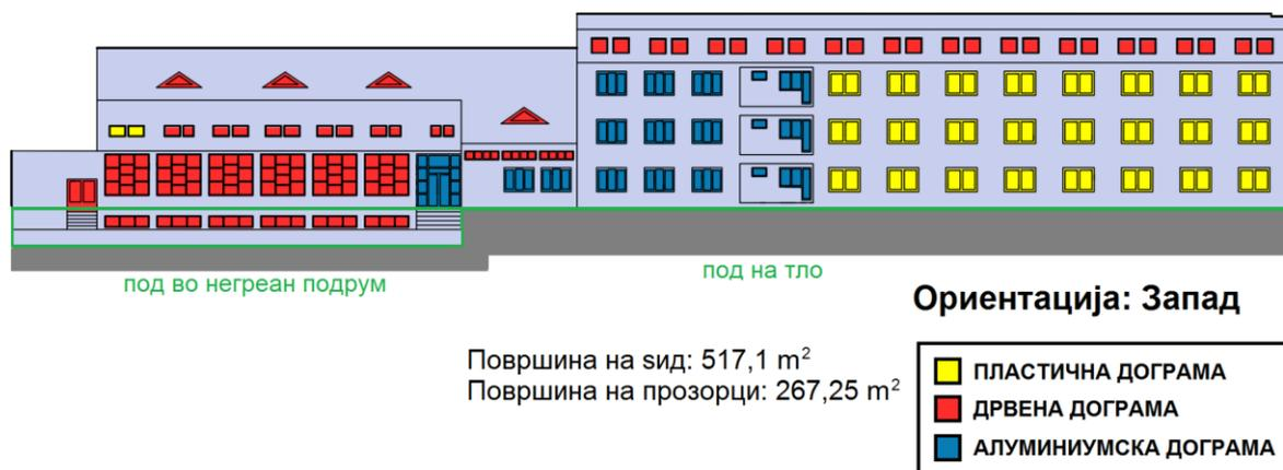
**Figure 3.** Dormitory's western façade – Total area without windows 517,1 m<sup>2</sup>; red colored windows are with double glazing and wooden carpentry; yellow colored are with PVC carpentry and double thermopan glazing with inert gas filling, while blue colored windows are with aluminum carpentry and thermopan glazing.
