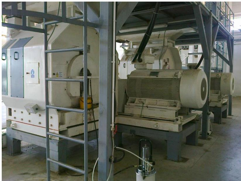
**Figure 4.** Machines for peletting of grinded straw
