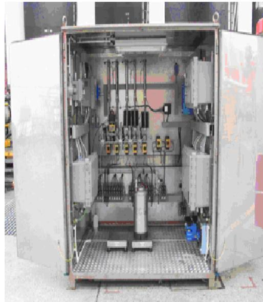
Figure 3. In-line sampler for sampling system
