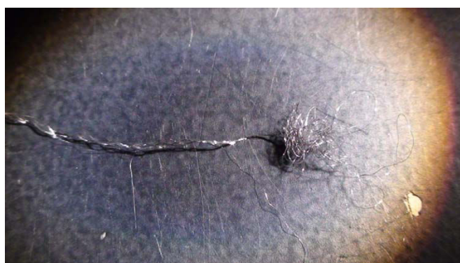
Figure. 3 Silver plated PA filament 36X enlargement (own photo)
