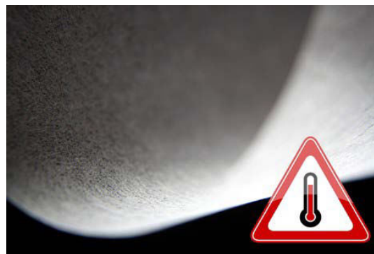
Figure 6 . Non-woven material for resistant on flamability developed by Technical Textile Products company. This material provides insulation from 500 to 1600°C
