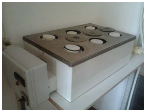
Picture 2 The measurement of water vapor permeability
