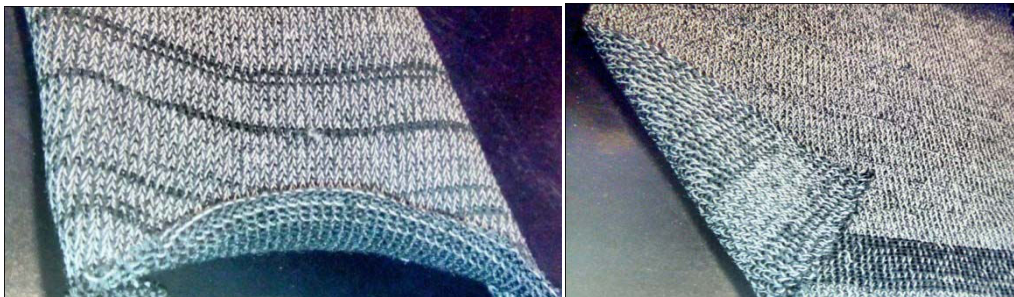
Figure 1 - Plated plain jersey (a) and plated rib (b) structures
