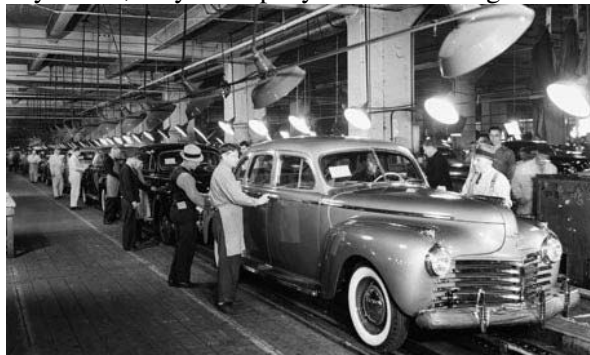
Figure 8: The workers making the final inspection on the finished models of the Chrysler Plymouth automobile
